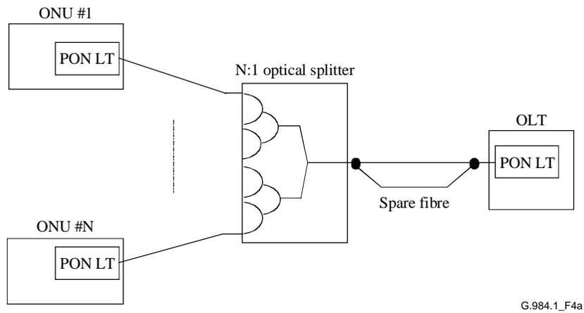
**Figure 4a/G.984.1 – Duplex GPON system: Fibre duplex system**
