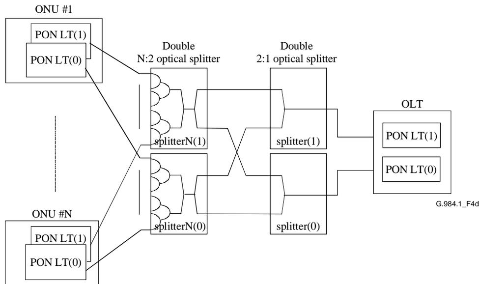
**Figure 4d/G.984.1 – Duplex GPON system: Partial duplex configuration**
