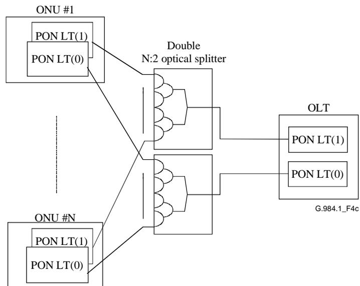
**Figure 4c/G.984.1 – Duplex GPON system: Full duplex system**
