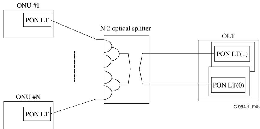
**Figure 4b/G.984.1 – Duplex GPON system: OLT-only duplex system**
